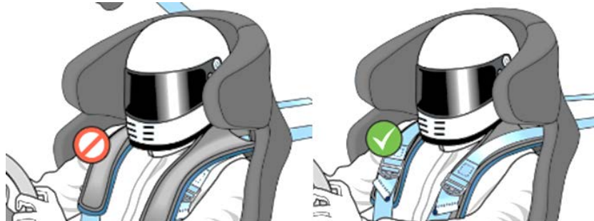
Figure 8 Example of incorrectly and correctly positioning of the harness straps when using a HANS®
